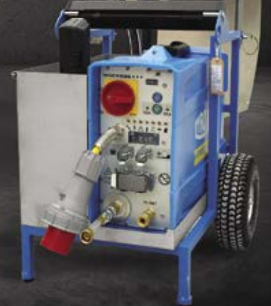
Complete Wall Saw Cart Assembly and Control Unit
