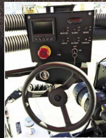
Digital Engine Panel, Fuel Gauge and E-Stop
