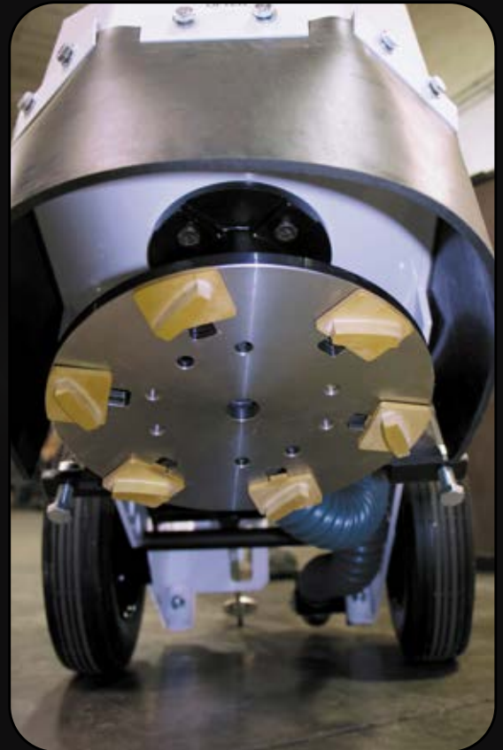
12" Grinding Plate Fits Diamond Products' CP200 grinders
