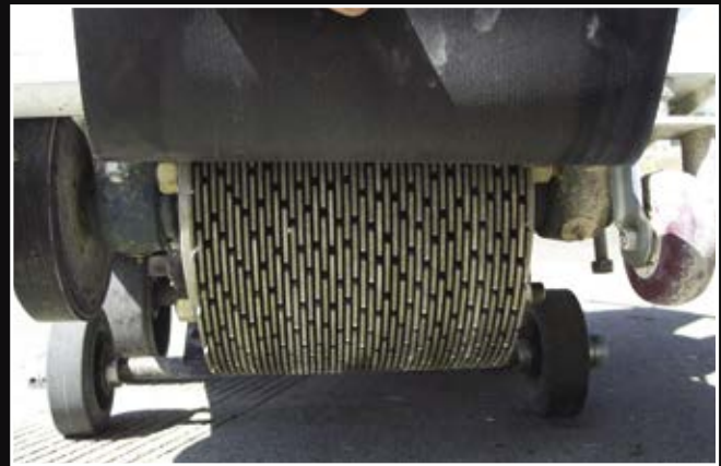
Uses 12" (30.48cm) diameter blades on a CG-1 10" (25.4cm) or CG-2 16" (40.64cm) grooving or grinding head with specifications that can be custom fit to your application
