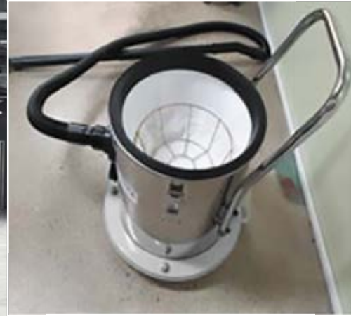
Pre-Filter for Dry Containment
