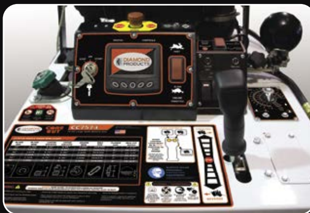
CC7574DD Control Panel
