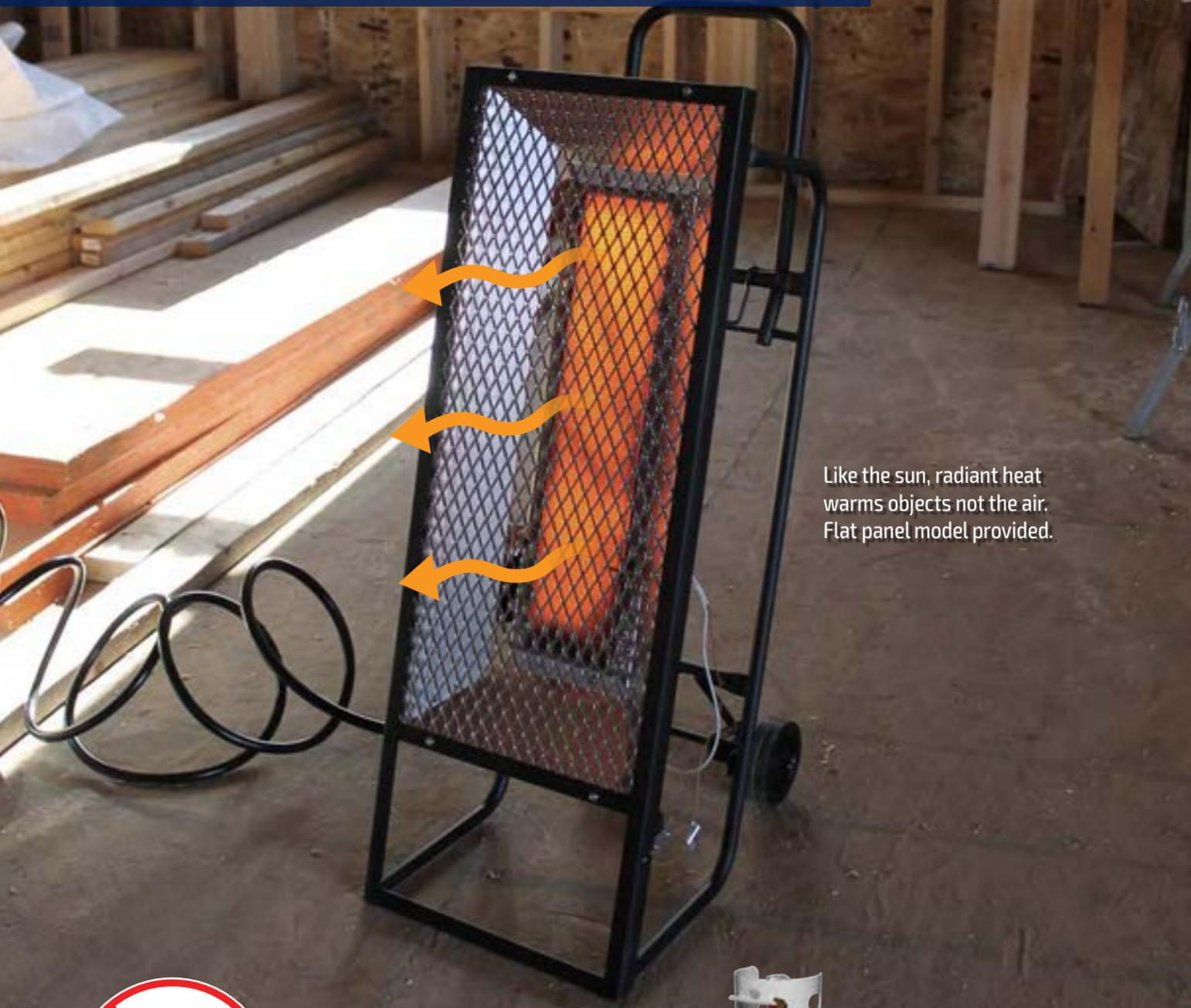
Like the sun, radiant heat warms objects not the air. Flat panel model provided.
