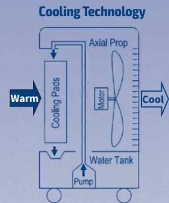
Water from an onboard tank is pumped to the top of a filter-like cooling pad. Then, a 3100 CFM fan pulls warm, environmental air over the filter and pushes out air with a cooling effect 30+ feet.
